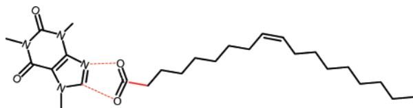
Figure 1. Bidimensional structure of caffeine oleate complex. The carboxylic acid...imidazole hydrogen bonding interaction of the caffeine oleate complex formation is indicated with dashed lines.
